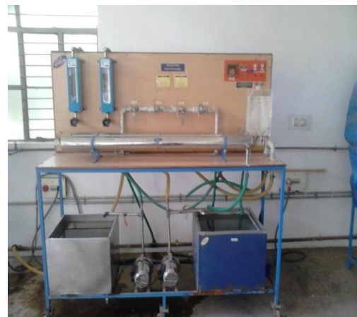
fig 1 Experimental setup of Double Pipe Heat Exchanger
